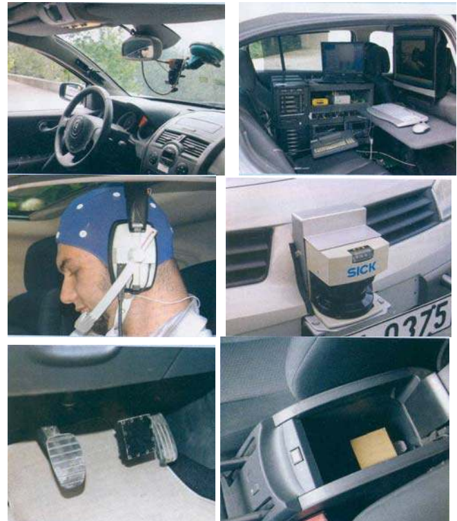
Figure 3. Sensors in the data collection vehicle upperleft clockwise: cameras, navigator area and lab bench for data acquisition systems, laser scanner, IMU XYZ accelerator, break pedal pressure sensor, headset/mics, and EEG cap.
