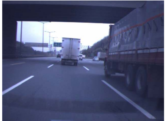
Figure 7. Laser Scan Reading and the photo for Driver IF1015 recorded at 12:56 PM on April 6, 2007. Truck on the right is between -200 to +800 cm, the white truck is away 22 meters, and the vehicle on the next lane (left) is about 23 meters ahead.
