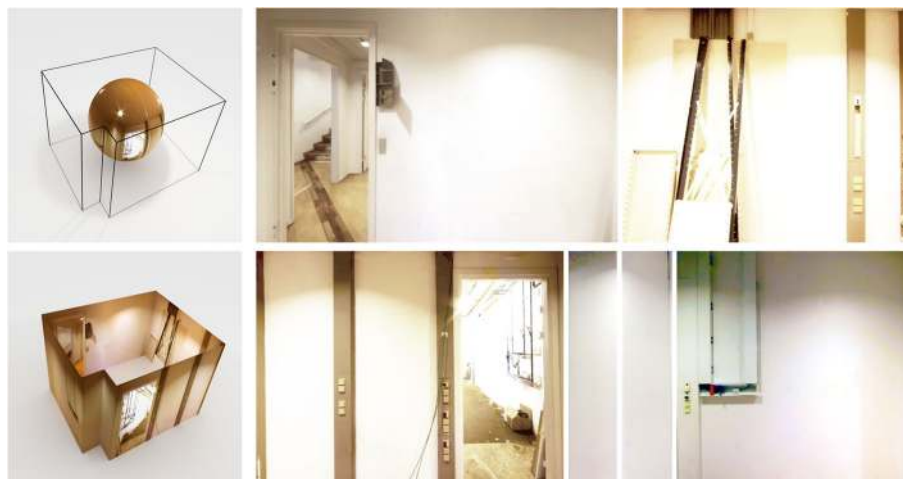
Fig. 7 Orthophoto generation. From the panoramic views and coarse wall geometry (left), orthophotos for each wall are generated (right)
