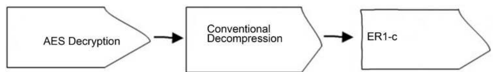
Figure 3. Decoding process of PMU data using ER1-c.
