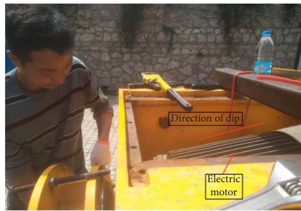
FIGURE 14: Motor mounting tilt.
