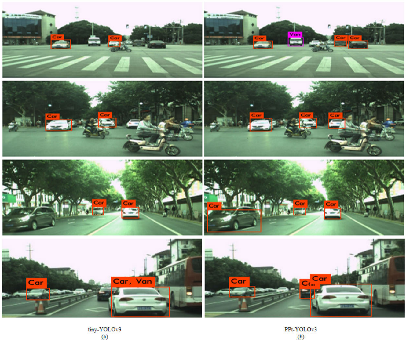
FIGURE 8. The comparison of detection results of images collected from roads with tiny-YOLOv3 and PPT-YOLOv3. Four pictures on the left were detected with tiny-YOLOv3, and four pictures on the right were detected with PPT-YOLOv3. A group of horizontal pictures are the same scene.
