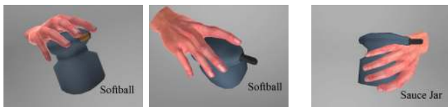
Fig. 24. Best hand poses for the sander. The first two softball grasps are the best among the five candidates (mug and softball grasps) considering the partial sander shape. The last grasp is the saucejar grasp, the best among the eleven candidates (saucejar, mug, and softball grasps) considering the whole sander shape.
