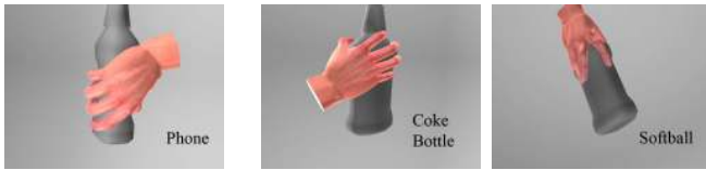
Fig. 23. Best hand poses for the mouthwash bottle. The first grasp (phone grasp) is the best among nineteen candidates (phone, jellyjar, cokebottle, and mug grasps) considering the partial mouthwash shape. The last two grasps are chosen from the sixteen candidates (phone, mouse, cokebottle, mug, and softball grasps) considering the entire mouthwash shape. The first one is a cokebottle grasp and the second one is a softball grasp.
