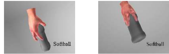
Fig. 26. Two softball grasp candidates with different metric values, caused by the difference in contact points.
