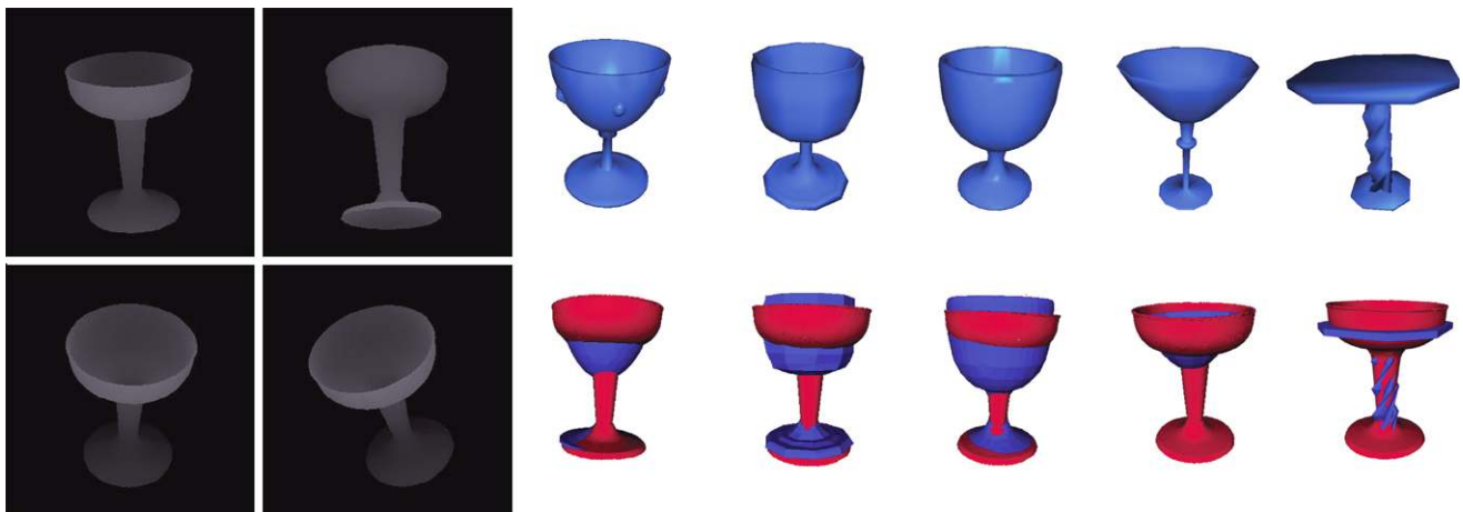
Fig. 7 (Color online) Alignment via matching Cap centers and refinement with ICP. Left , depth images of a wineglass, using a NextEngine laser scanner. Top right , five matching models from the database. Bot-
