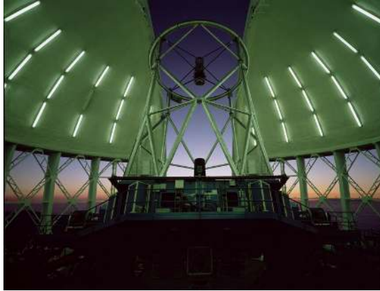
Figure 1.1: Gemini North telescope with open wind vents and observing slit. Gemini North is a 8m telescope located on Mauna Kea, Hawaii. Image Credit: Gemini Observatory / Association of Universities for Research in Astronomy.
