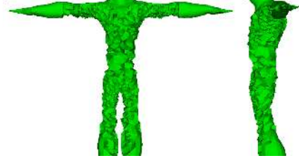
Fig. 4. VSMPL layer obtained for the higher resolution mesh (3.5 times more nodes and 5.4 times more elements).
