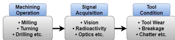
Figure 18. Generalized direct tool condition monitoring method
