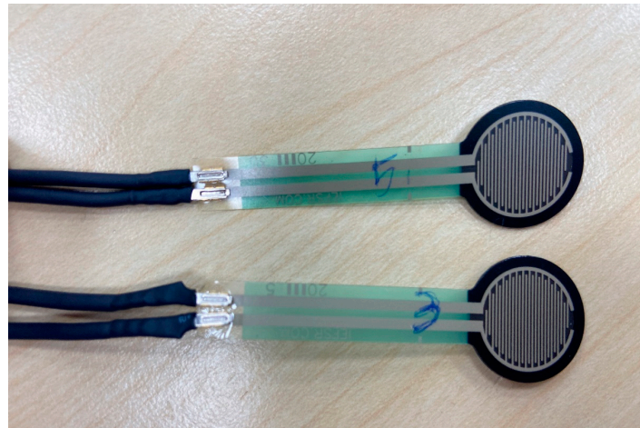
Figure 4. FSR resistor-based force sensor.
