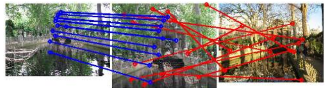
Figure 3: Example of image matching using the SIFT descriptor. While SIFT works very well at matching fine image structure (left), it fails miserably when there is too much local change, such as a change of season (right).
