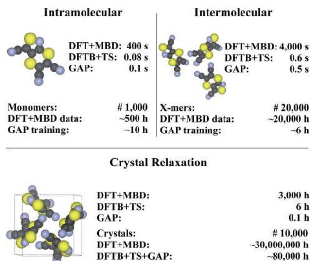
Fig. 7 Timings for generating the (intra- and intermolecular) model for XXII and crystal relaxations (as obtained on a Intel® Xeon® CPU E5-2697 v3 @ 2.60 GHz processor). The upper part in each of the tree sections illustrates timings for a single unit (monomer, X-mer or crystal), while the lower part corresponds to the time required for the specified number of training configurations (top) and an exemplary number of crystal relaxations (bottom). The costs for relaxations are included in the intramolecular timing (see text). Values are rounded to one significant digit (both in terms of time and number of geometries). For details see ESI.†
