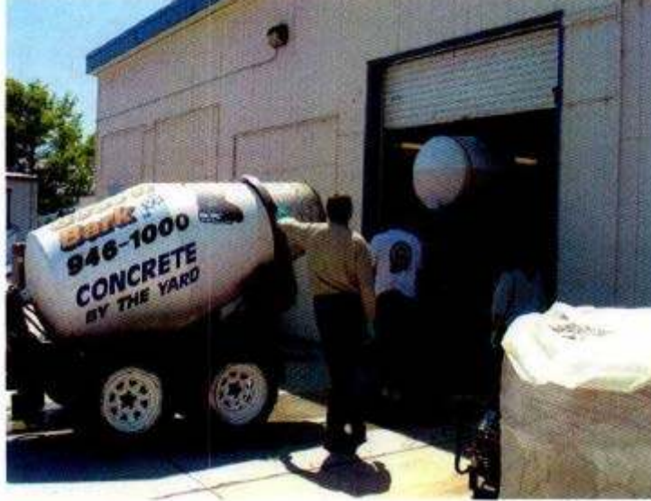
Figure 4.1. Portable Cement Mixer Used to Create the Cubic Meter Cast Stone Waste Form. See Figure 4.4 for photograph of Cast Stone Block (covered by ammonia gas-collection system).
