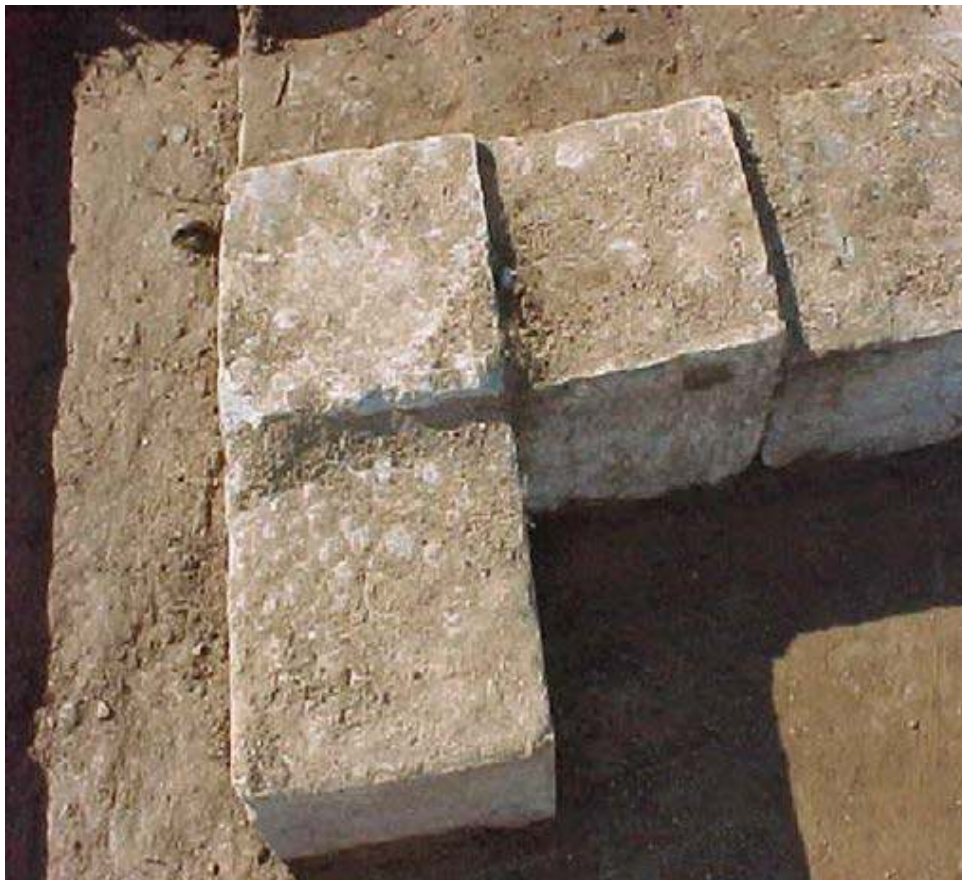
Figure 6.2. Cement Waste Forms after 39 Years of Shallow Burial (see Sobolev et al. 2006)
