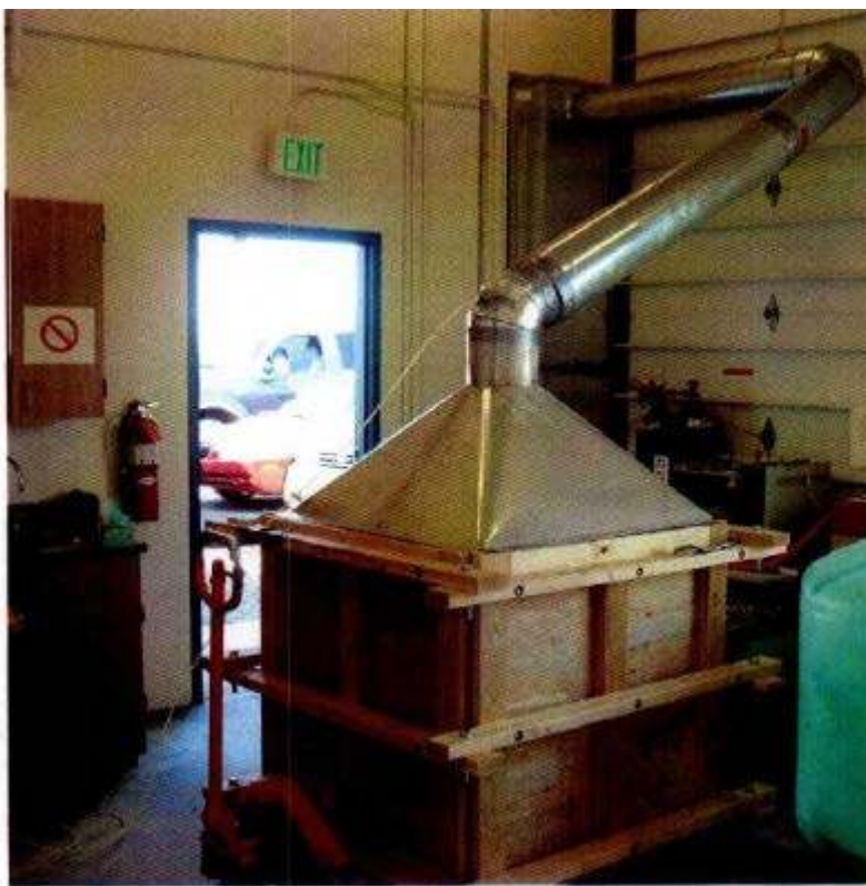
Figure 4.4. Cast Stone m 3 Monolith (wooden box used to support mold and with ammonia gas collection system emplaced right above the monolith) from Cooke et al. (2006a)
