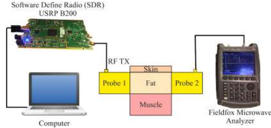
Fig. 6. Received signal strength measurement setup.
