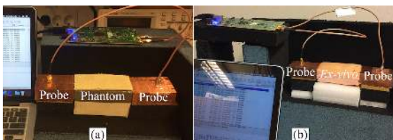
Fig. 8. Experimentation setup in (a) Phantom and (b) Ex-vivo environments consisting of skin, fat, and muscle layer.
