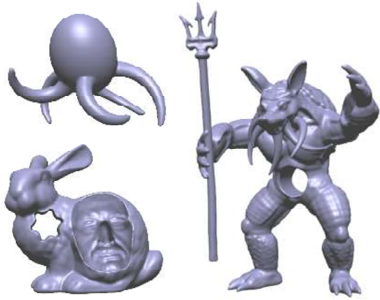
Fig. 6: Free form deformation and boolean operations. Top left: several tentacles are pulled out from an ellipsoid. Bottom left: a hole and a face mask are created on the bunny's surface. Right: an interesting creature is created from the armadillo using free-form deformation and boolean operations.
