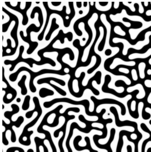
Figure 2: A visualisation of a 512x512 two-dimensional Cahn-Hilliard field at t = 131072 .
