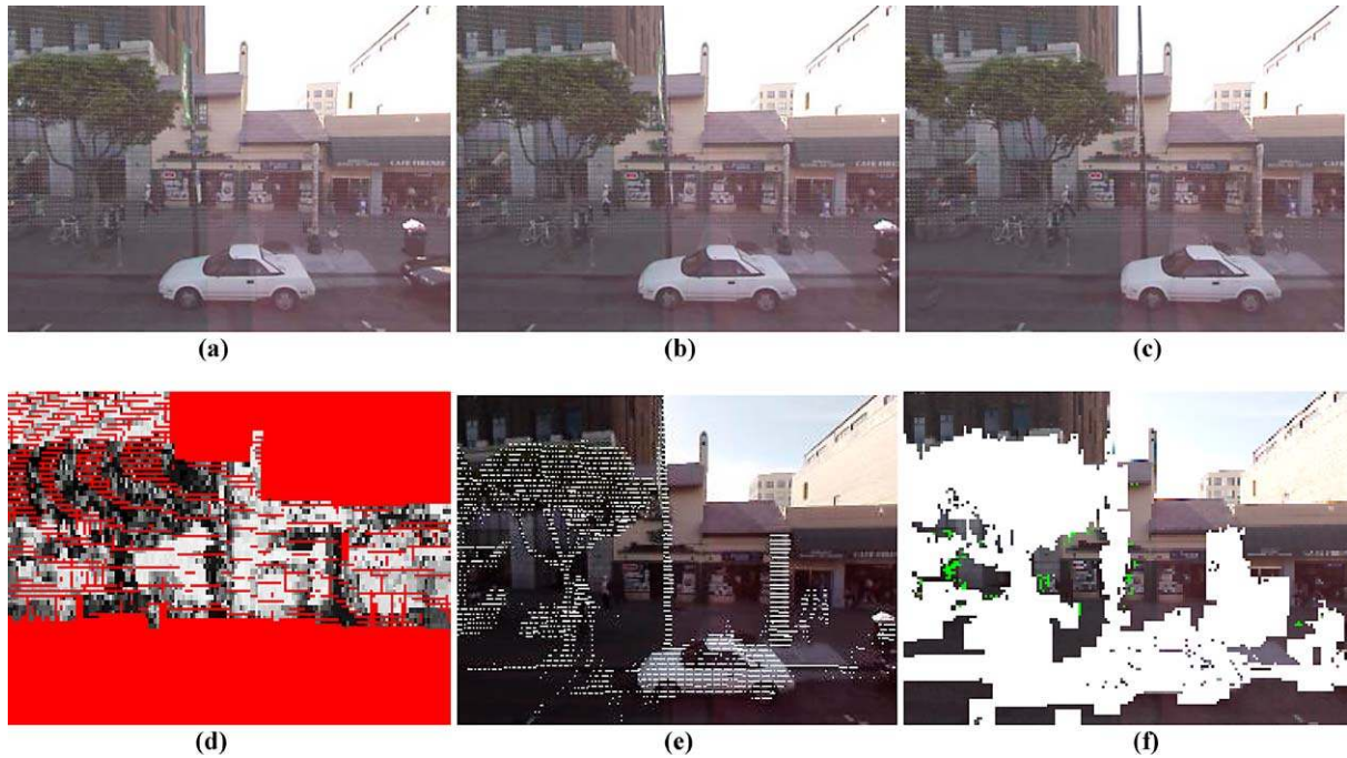
Figure 21. (a), (b), (c) sequence of three camera images I_{c-1} , I_c , I_{c+1} . (d) correspondence error for I_c shown as gray values. White corresponds to low value and black corresponds to high value of \varepsilon . Red pixels are pixels where no background scan points projected. \varepsilon is not computed at these pixels. (e) Foreground scan points marked as white pixels. (f) Foreground regions of I_c marked as white, using color constancy and correspondence error. The green triangles are the triangles used for texture mapping/atlas generation from this image.
