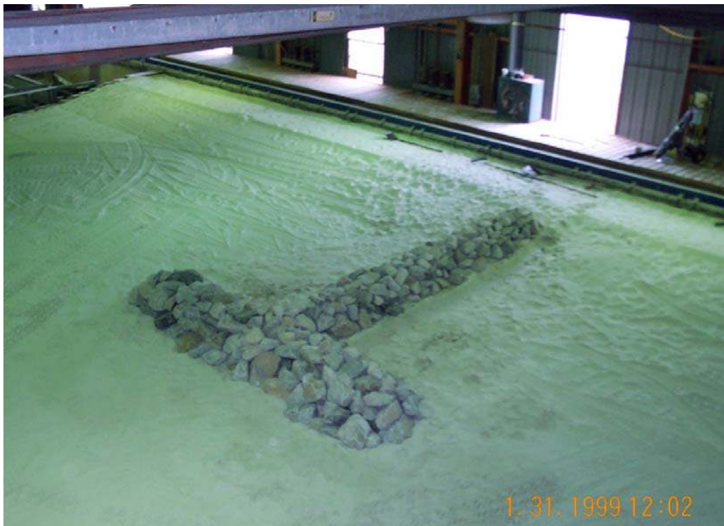
Figure 113. Completed T-groin structure in LSTF model beach.
