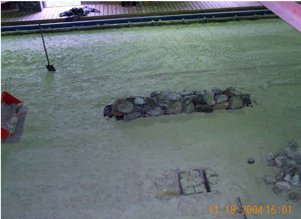
Figure 144. Completed nearshore breakwater structure in LSTF model beach.
