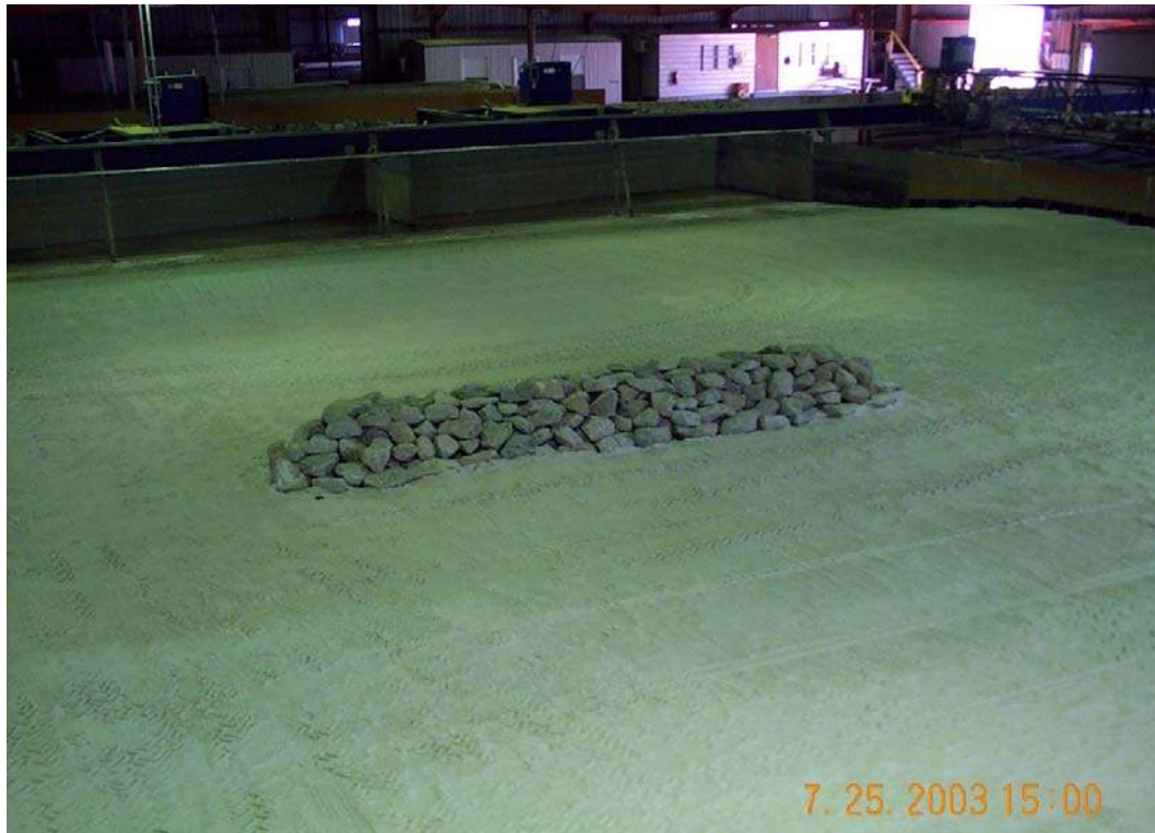
Figure 30. Completed breakwater structure in LSTF model beach.
