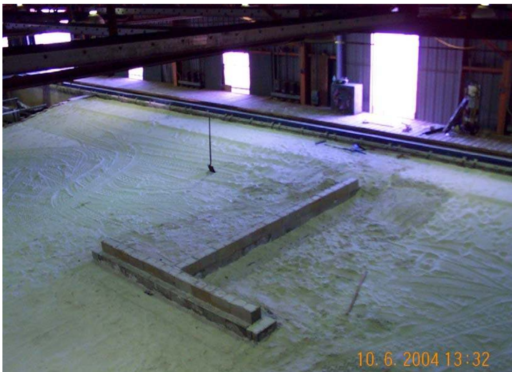
Figure 112. Third layer concrete block T-groin core.
