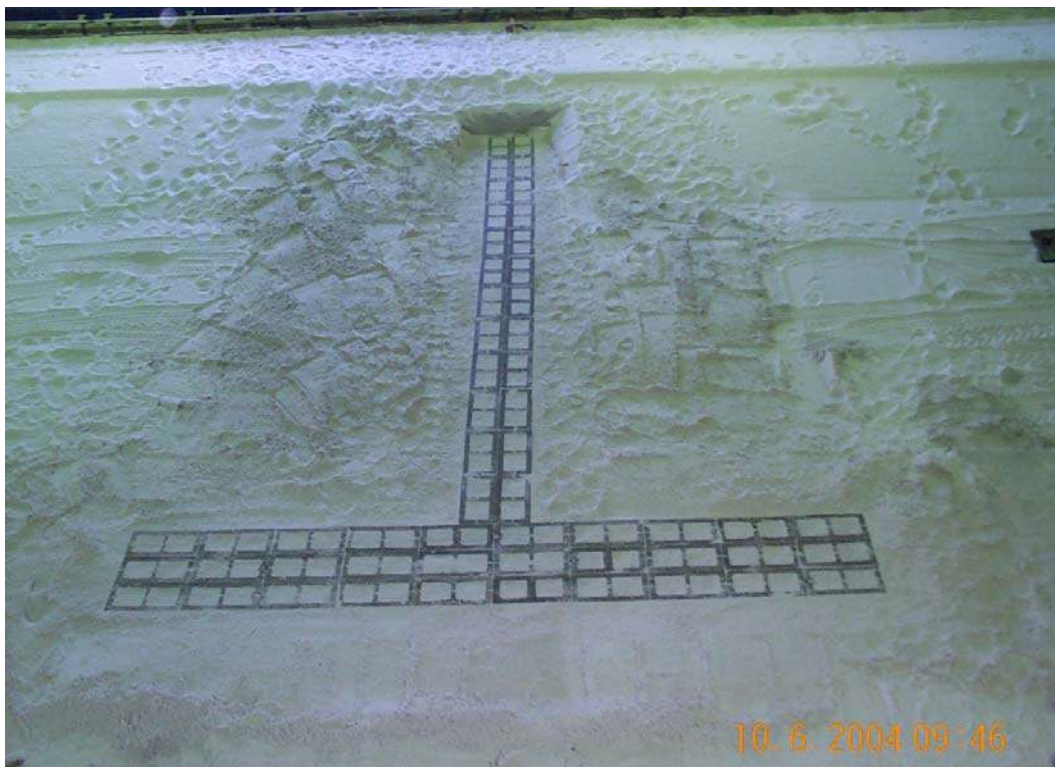
Figure 110. T-groin foundation backfilled with sand.
