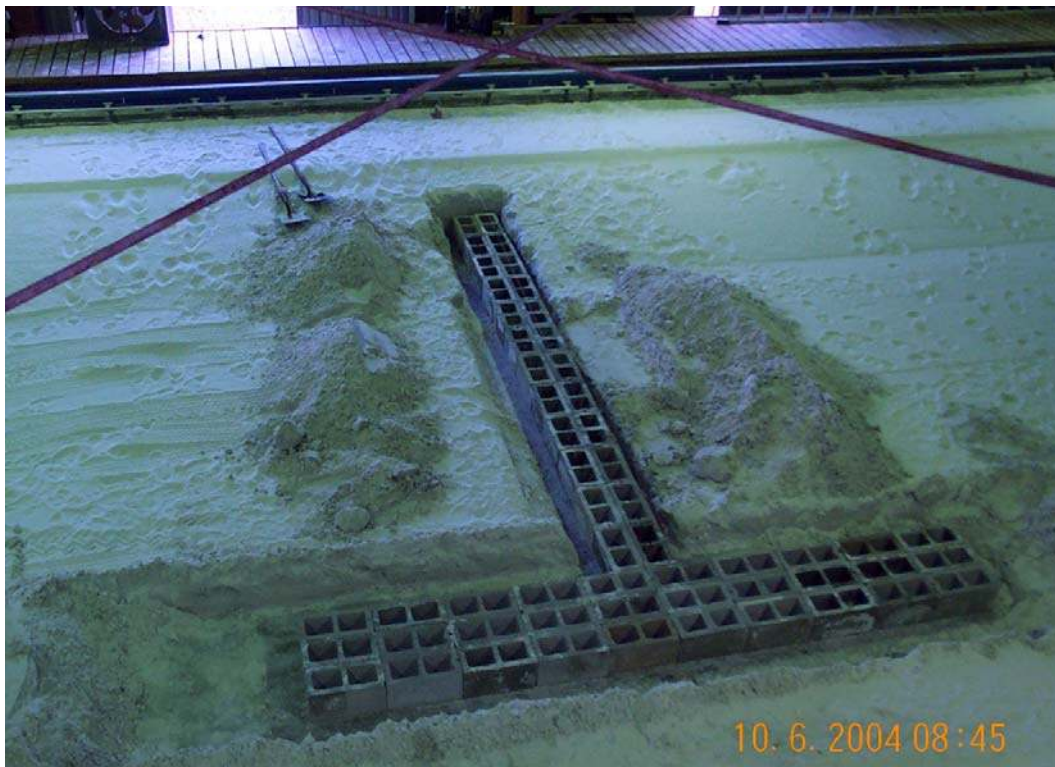
Figure 109. T-groin foundation and core.
