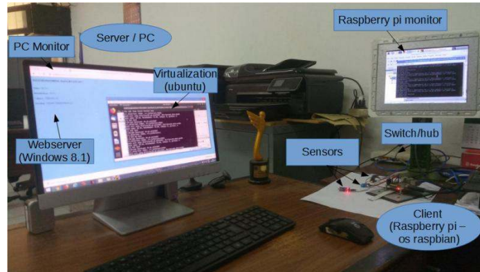
Figure 9. Hardware of the room condition telemonitoring application
