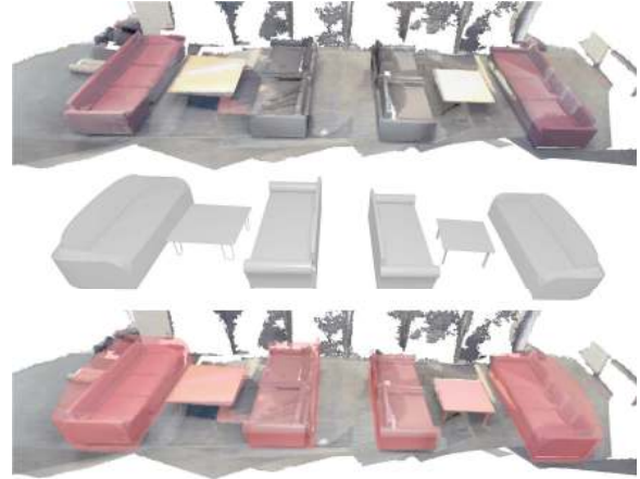
Figure 9: Results on a scanned scene of couches and tables. From the scene (top), couches and tables are identified and registered to (bottom), resulting in a clean reconstruction of the scene with high-quality geometry (middle).
