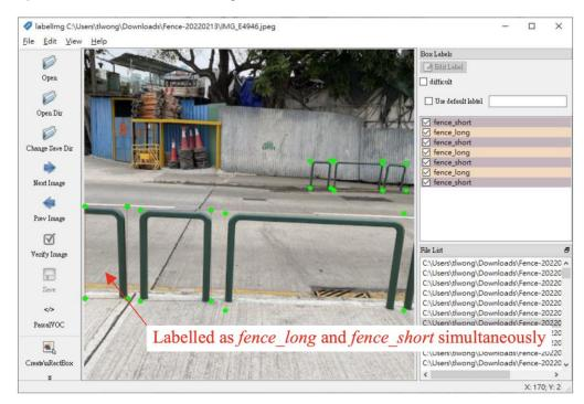
**Figure 5.** Example of labelling partially out-of-view objects. A partially out-of-view object was labelled as *fence\_long* and *fence\_short* simultaneously since it cannot be classified by a single image.
