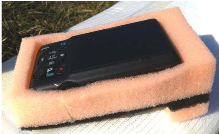
Fig. 9. The instrument for Stable Placement of ONboard Gear and Equipment (iSPONGE), which is installed in the Conservation Drone to avoid vibration blur in photographs.
