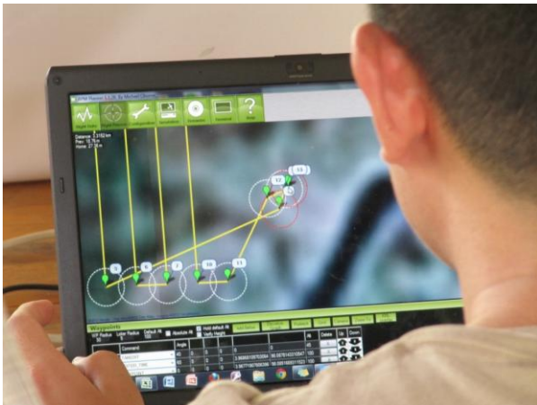
Fig. 2. APM Planner software used to plan the flight paths of each drone mission.
