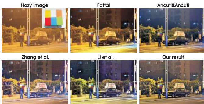
Fig. 10. Comparative results on the image with color checker provided by Zhang et al. [18]. The night-time hazy image with color palette (top-left) is enhanced by several dehazing techniques. See Table IV for the PSNR values.
