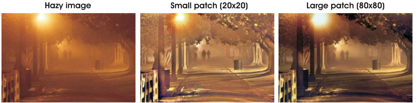
Fig. 6. Our experiments reveal that using a small patch size (e.g. 20 \times 20 on an image of size 800 \times 600 ) gives the capability of adjusting the airlight estimation to the local light source(s). However, by compensating local illumination, such a small patch also results in an important loss of global contrast and chroma. This limitation is solved by using a larger patch (e.g. 80 \times 80 for an image of size 800 \times 600 ), which considerably improves the global contrast by maintaining a consistent airlight estimate over the entire scene. Our work proposes to improve the performance by using both of patch size alternatives, by merging the two images reconstructed from a small and a large patch size.
