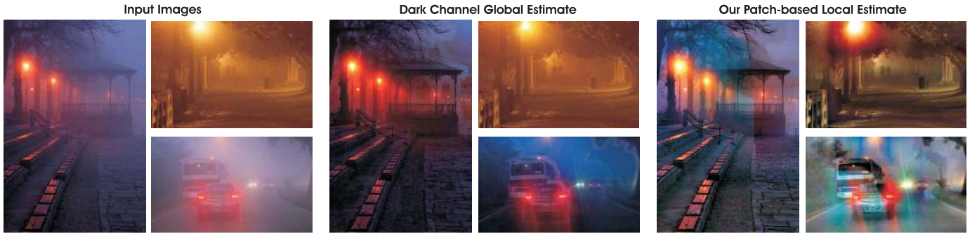
Fig. 2. Importance of local airlight estimation in night-time scenes. Designed for day-time dehazing, the well-known dark channel [37] has important limitations on night scenes because it assumes a spatially constant airlight. As may be observed in the last column, our patch-based local estimate (also not refined) of the airlight is more appropriate for night-time hazy scenes. In particular, color and details that are close to light sources are better enhanced.
