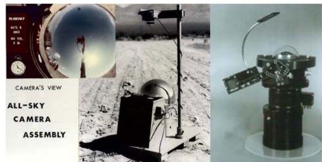
Fig. 1. (Color online) Two early WSI systems developed at MPL, the all-sky camera used in 1963, and the digital day WSI used in the 1980s.
