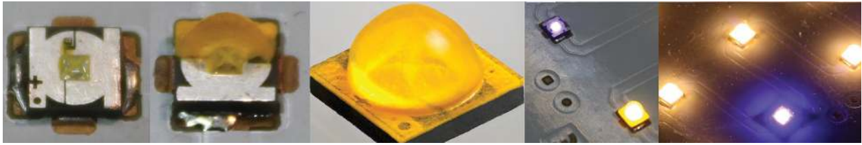
Figure 1. High power 3000 K white XTE LED by CREE. Blue emitter with phosphorus cover.
