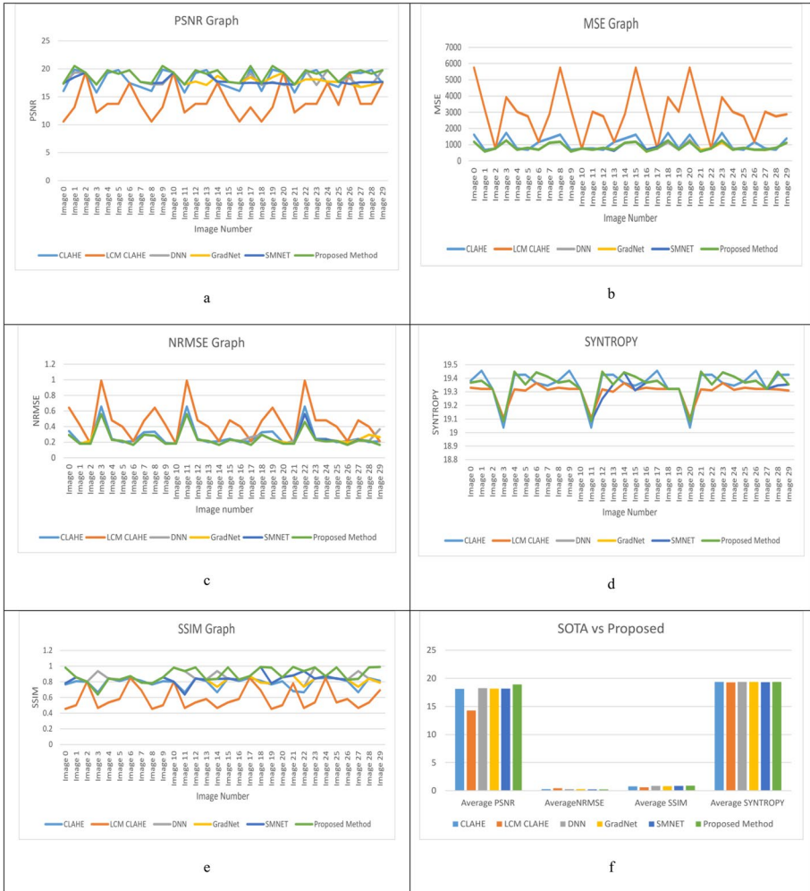
Fig. 10 Comparative graphs of CLAHE, LCM CLAHE, and DBST LCM CLAHE, a : Graph of PSNR, b : Graph of MSE, c : Graph of NRMSE, d : Graph of Entropy, e : Graph of SSIM, f : Graph of SOTA vs Proposed
