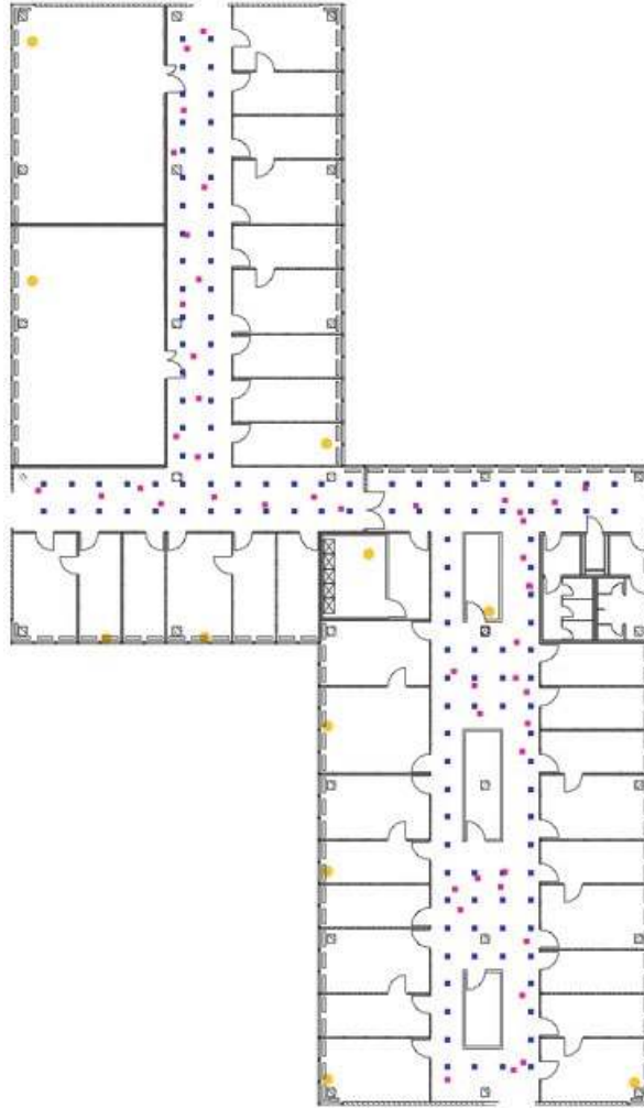
FIGURE 6: Floorplan of the testing area in the dataset used for evaluation. The red dots show the locations where online RSS observations are collected, and the blue dots show the offline observing locations. Yellow dots show the locations of the APs, which we do not assume to be known in our experiments.
