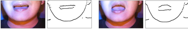
Figure 12: Lip contour extraction using two red and blue lights placed above and below the camera.
