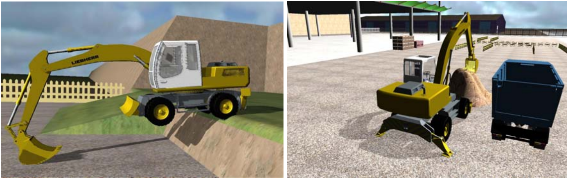
Figure 7: Using the arm for descending a steep slope and terrain excavation.
