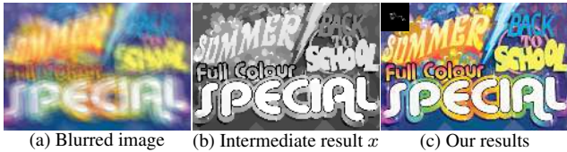
Figure 6. An example with complex background regions. The size of estimated kernel is 99 \times 99 pixels.
