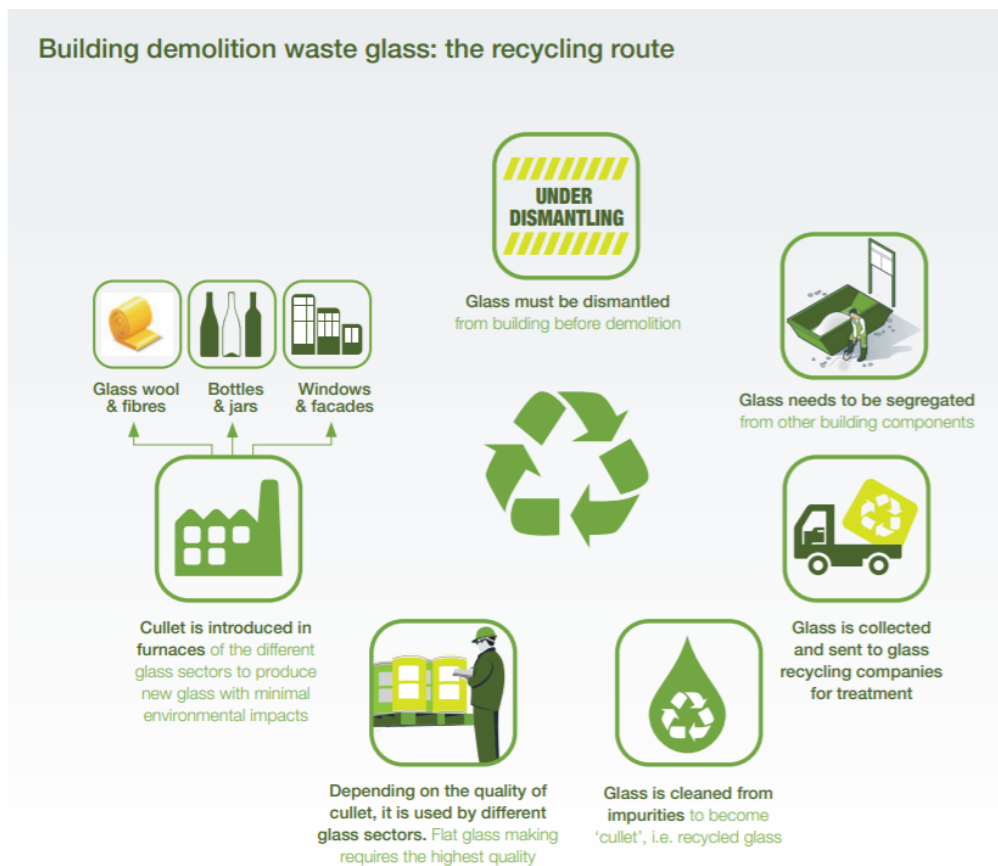
Figure 12: The recycling pathway for demolition waste. Source 280
