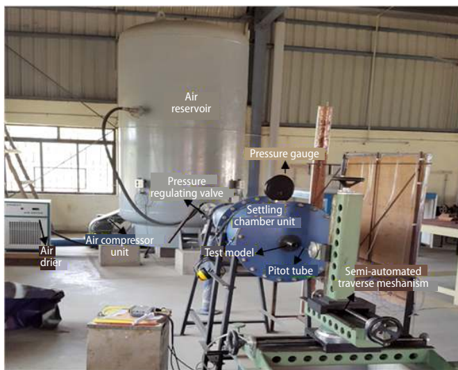
Figure 4. Free jet facility at high speed jet laboratory of Rajalakshmi Engineering College
