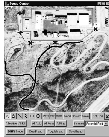
Fig. 11. Base station control window. The initial positions of the vehicles were at the lower left corner of the screen. The vehicles first follow their assigned paths. Once they reach the end of their paths, the vehicles use the obstacles and attractors to navigate to their final positions on the goal attractors. To avoid collision between the vehicles and to uniformly cover the goal attractors, the vehicles are also repulsed by each other. The obstacles are drawn in red, the goals are drawn in green, and the vehicle paths are drawn in black.
