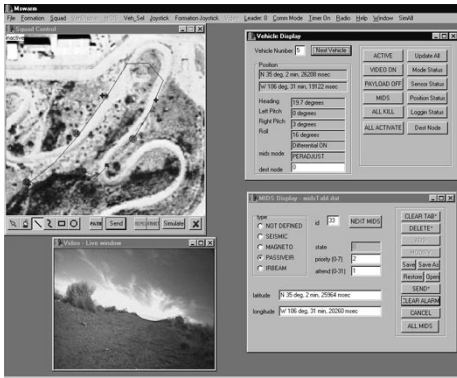
Fig. 8. Base station's GUI displays vehicle status, remote sensor status, video, and GPS position on a GIS map.
