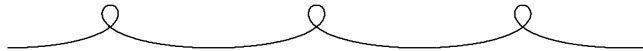
Figure 5.1: For a UAV orbiting a moving target, the trajectory exhibits loops corresponding to the times when the UAV and the target are moving in opposite directions and long arcs when both are moving in the same direction.
