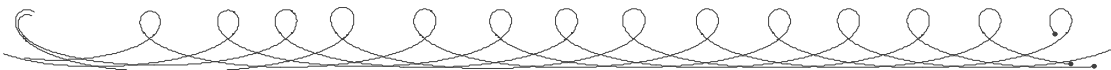
Figure 5.7: Trajectories of 4 UAVs orbiting a moving target trace out routes similar to those in this figure.
