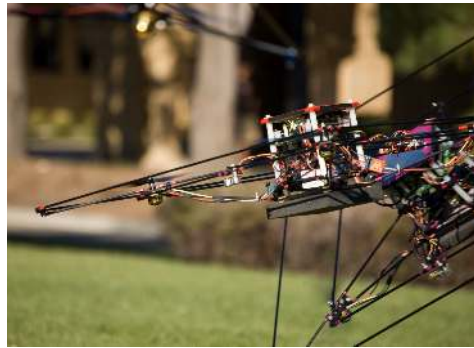
Fig. 1. A mid-air collision between two out of three remote-piloted quadrotor helicopters operating in close proximity. The proposed algorithm would assume control when required to prevent imminent collisions.
