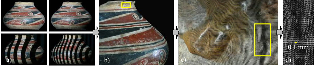
Figure 3. Photogeometric Capture System. a) Our method captures photometric (top) and geometric (bottom) observations of an object. b) A novel viewpoint rendering of a 3D model is produced using our photogeometric method. c) A close-up of the model rendered with texture mapping. d) An even closer view of the model now rendered using wireframe and synthetic shading showing details beyond those possible using only geometric observations. Our approach uses the same hardware as standard structured-light but is fully self-calibrating and able to capture models at the resolution of the camera (in this example camera resolution is 10x greater than projector resolution). The average triangle edge length is 0.09035 or about 0.1 mm.
