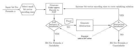
Fig. 1. Abstraction-based approach to solving bit-vector arithmetic
