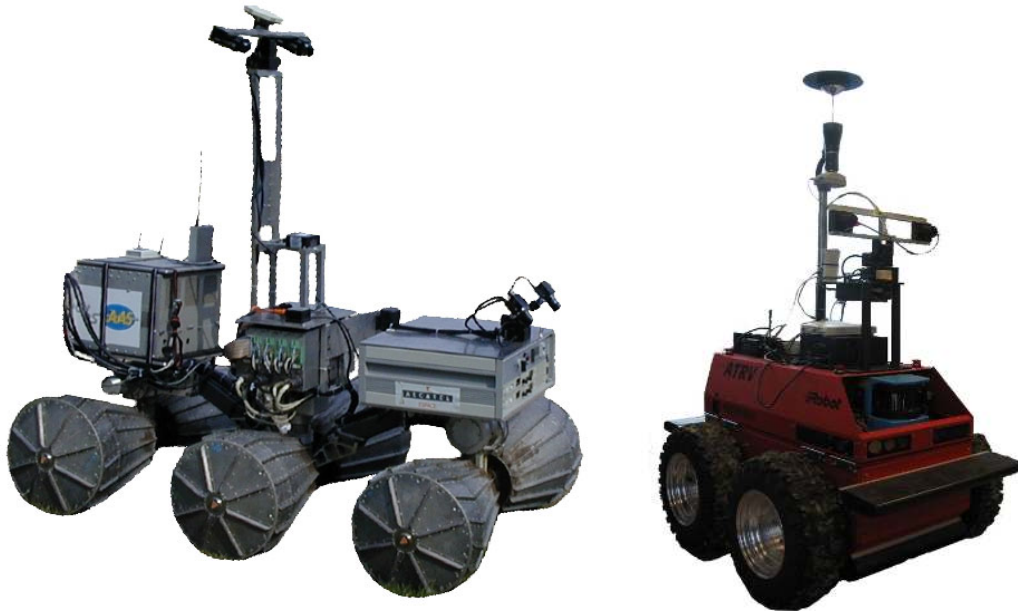
Fig. 1. The two rovers Lama and Dala, fully equipped with on-board sensing and processing capabilities.
