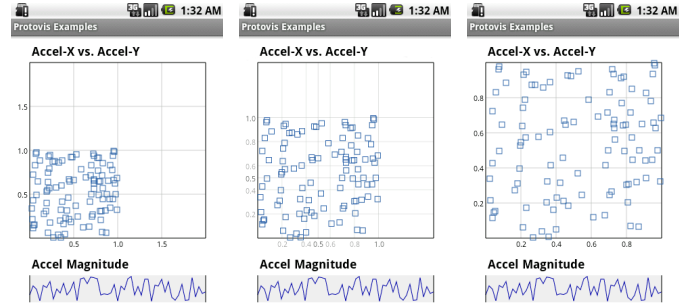
Fig. 8: Protovis on an Android mobile phone. The image sequence shows a touch-initiated animated scale transition in a scatter plot.
