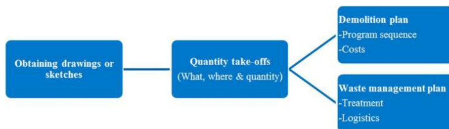
Fig. 1 Traditional demolition process
