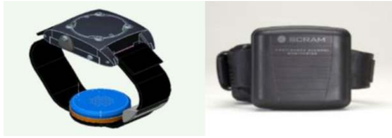
Figure 7.1: Alcohol Biosensor Devices: Left panel: The Giner WrisTAS. Right panel: The AMS SCRAM.
