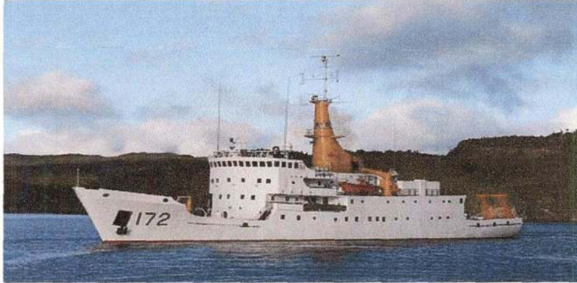
Fig. 7. The Quest is specifically designed for open ocean acoustic research. The vessel is equipped with an ultra quiet turbine drive system to preserve the low-noise environment required during sensitive measurements [8].
