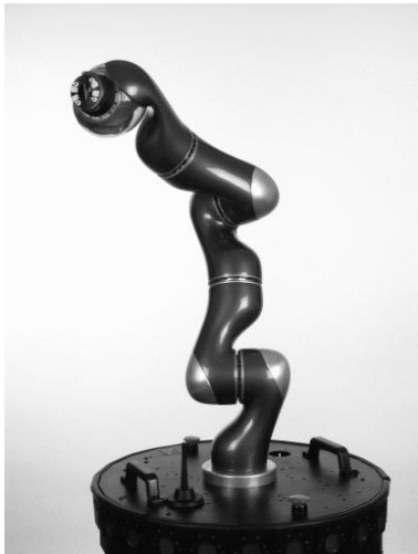
Fig. 5. 7DOF DLR-light-weight-robot (third generation)
