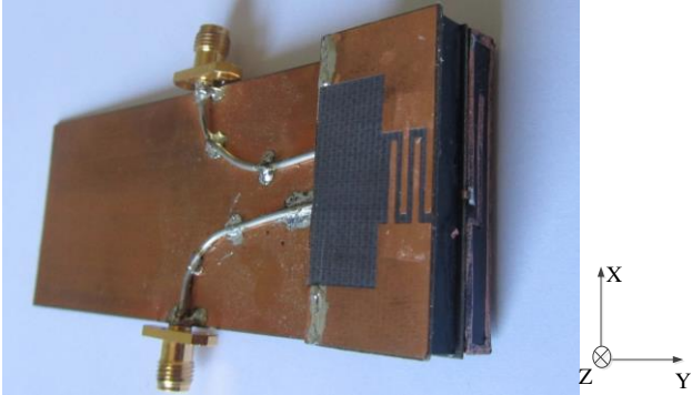
Fig. 15. The prototype of the co-located dual-antenna system, consisting of the folded monopole and the coupled loop.
