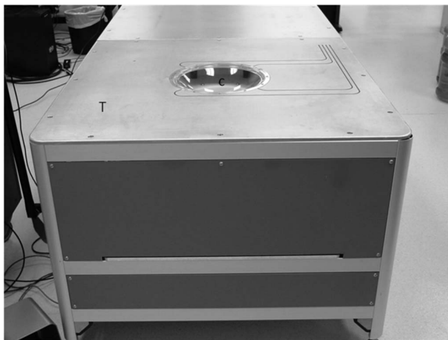
FIG. 1. Photograph of PAM scanner showing the exam table (T) and the breast positioning cup (C), below which is located the hemispherical detector array.
