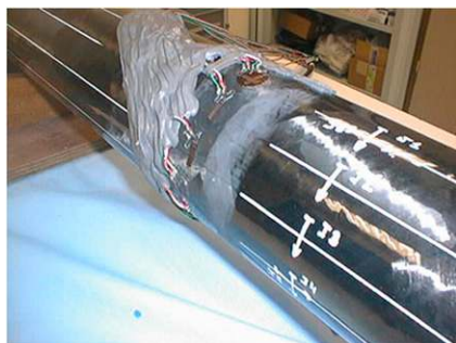
FIG. 7. Testing the tube in the pressure tank. (left) Before the test the tube is fitted with strain gauges stuck around the hull. (right) During the test deformations of the gauges are measured ( \mu strain) while pressure cycles are applied by the pressure tank for 3 days.
