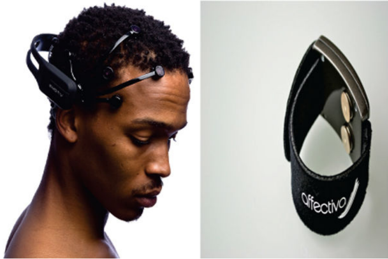
Fig. 4. Emotion measurement technology: (right picture) Affectiva by MIT's Media Lab works based on facial cues or physiological responses; (left picture) Emotiv by Emotive Systems is an Australian electronics company developing brain-computer interfaces based on electroencephalography (EEG) technologies. We thank Emotiv Inc. and Affectiva for their permissions to use their images.
