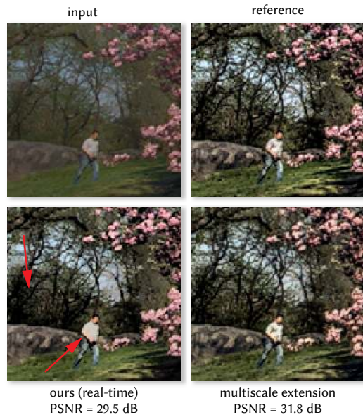
Fig. 13. At the expense of extra computation at full-resolution, our model can be extended with richer affine regression features. Here, by using a 3-level Gaussian pyramid as features \phi , we can better capture the high-frequency details in the the Local Laplacian (strong) task.
