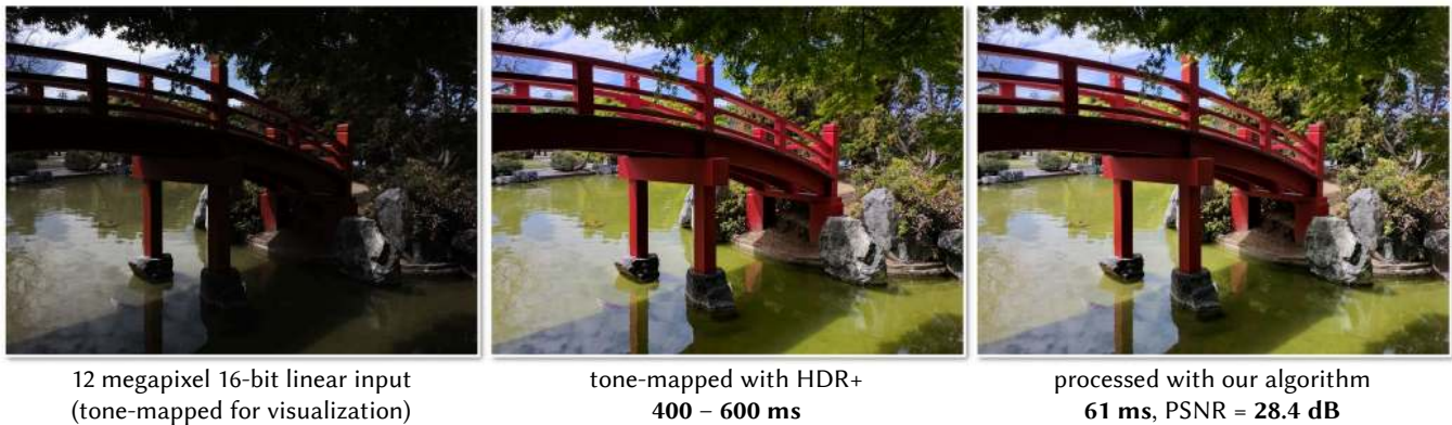
Fig. 1. Our novel neural network architecture can reproduce sophisticated image enhancements with inference running in real time at full HD resolution on mobile devices. It can not only be used to dramatically accelerate reference implementations, but can also learn subjective effects from human retouching.
