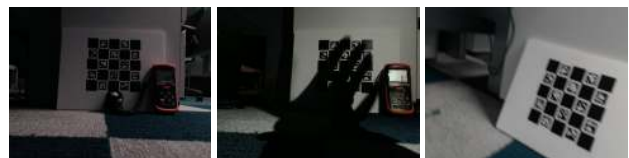
Figure 7. ChArUco Evaluation Set. Examples of frames from the ChArUco evaluation set. From left to right, each frame focuses on lighting (10lux), shadow, motion blur.
